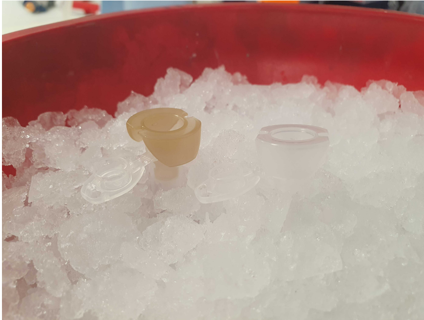
Figure 1. 2 mL Eppendorf tubes with 100 \mu m filter (brown, left) and 70 \mu m filter (white, right).
