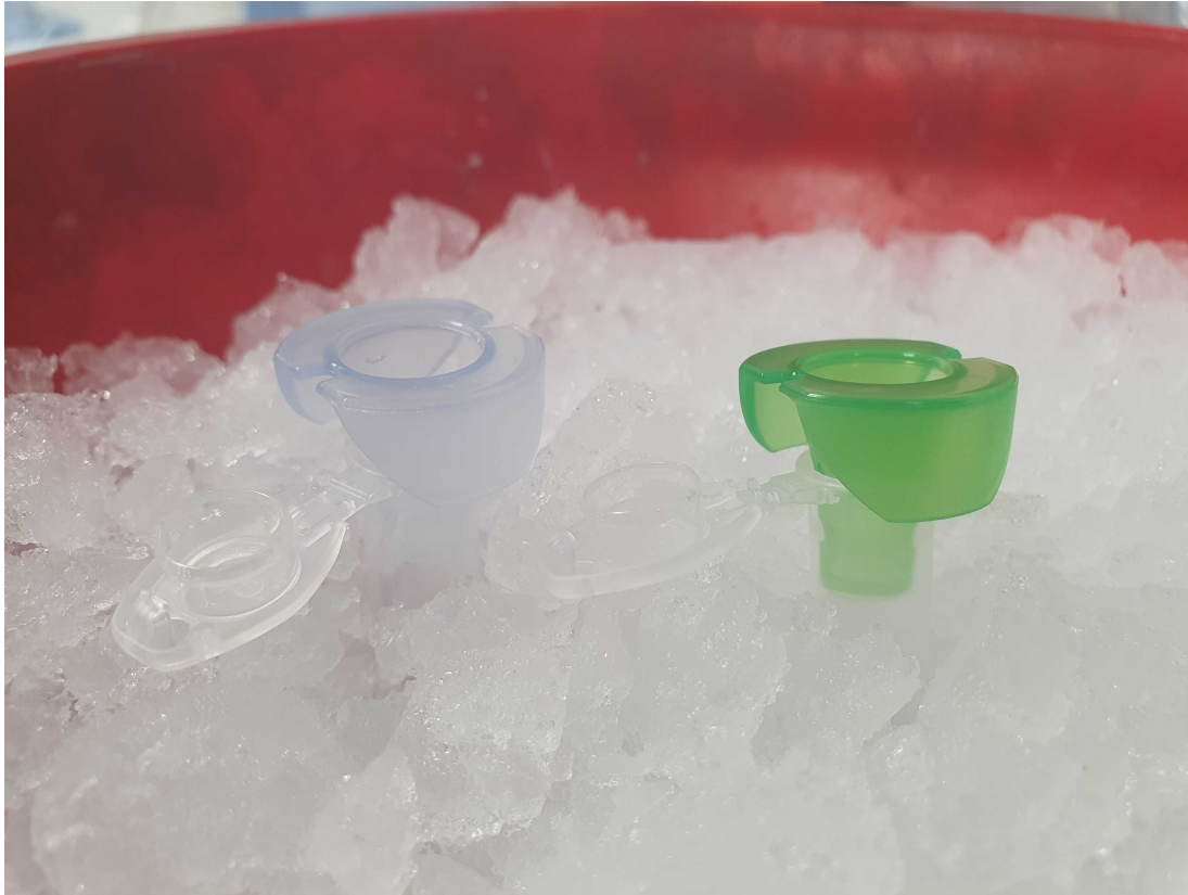
Figure 2. 2 mL Eppendorf tubes with 40 \mu m filter (blue, left) and 20 \mu m filter (green, right).
